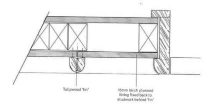
Curved timber wall detail in section & plan
